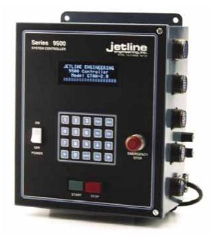
An important advantage of the 9500 Controller, compared with more conventional units, is that it employs a menu system to create weld programs through the keypad. Actual values can be entered and are displayed. This permits the parameter levels to be pre-selected before welding starts. During welding, the display provides a readout of actual weld values.
