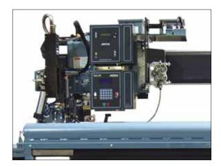
When ordered and supplied with standard firmware, the 9500 Controller permits all four channels to be programmed. A weld program can be made during which the welding current can be programmed for initial current, upslope, weld current, taper, downslope and final current levels. The weld can be time based or the weld length can be controlled by an external signal, a limit switch or an encoder. The operator can start downslope at any time, if required.
